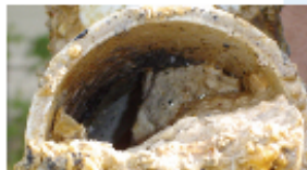
Pouring fat, oil and grease down the sink can lead to blocked sewers
