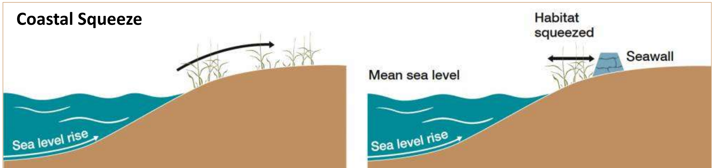
Diagram showing how the presence of coastal defences can lead to coastal squeeze and the loss of intertidal habitats
